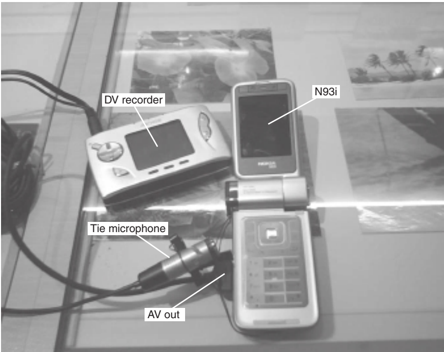
Figure 10.5 The recording apparatus. In this configuration, the synchronization of outgoing and incoming audio is made within the DV recorder.
